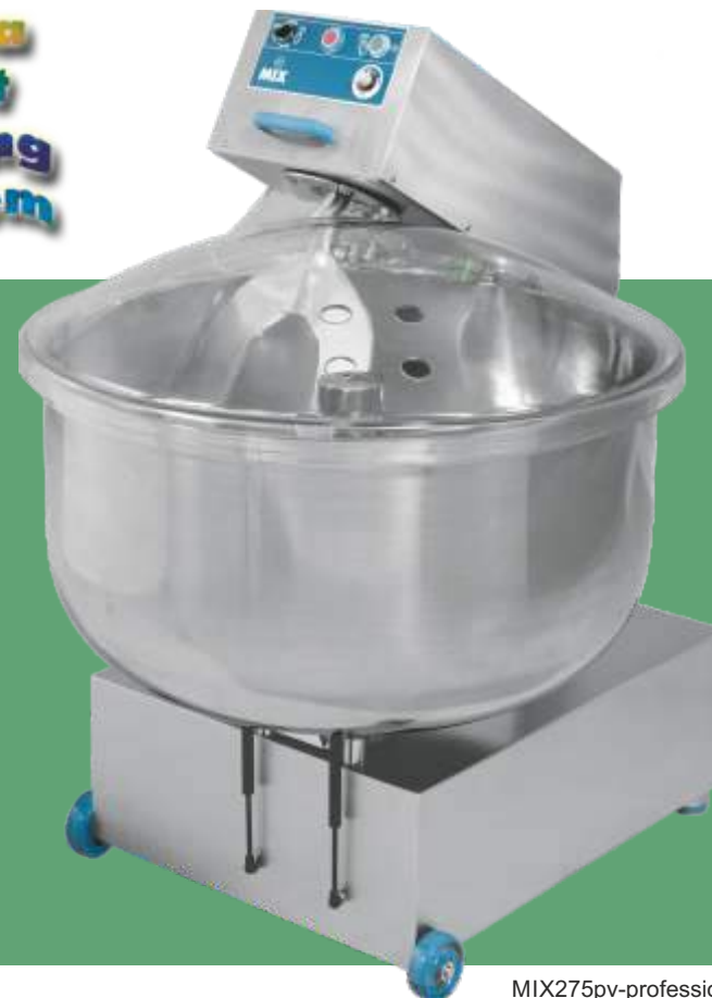
MIX275pv-professional, 2 motors, optional V-electronic variable blade speed
